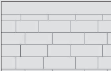
LINEAR PATTERN WITH 100% 180mm TANDEM UNITS.
